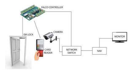
First, check Navigator IP Address and Port number by clicking System setting from Navigator Software. These will be used later by the Falco system.
