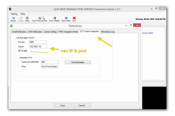
Enter Navigator IP address and port number. Make sure to tick the "Enable" option.
