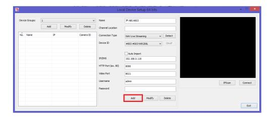
3. Once the camera stream of the Navigator Enterprise or Corporate is added, you can drag-n-drop the camera stream into Navigator Client.
