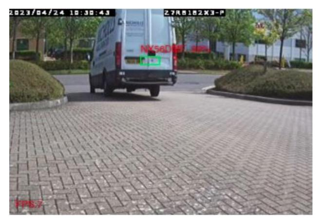
This is triggered when a vehicle enters the target area. If LPR allowed is selected then for an alarm/event the number plate must be in the cameras allowed plate list
