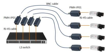
Caution: Do not use LILIN PoE switch connect directly to PMH-IP01 BNC-to-IP convertors.
