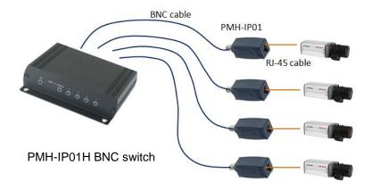
Caution: PMH-IP01H with BNC male terminators at channel 2, 3, 4, do not remove the terminators if you do not use these channels. It will cause PMH-IP01H switch not working properly.
