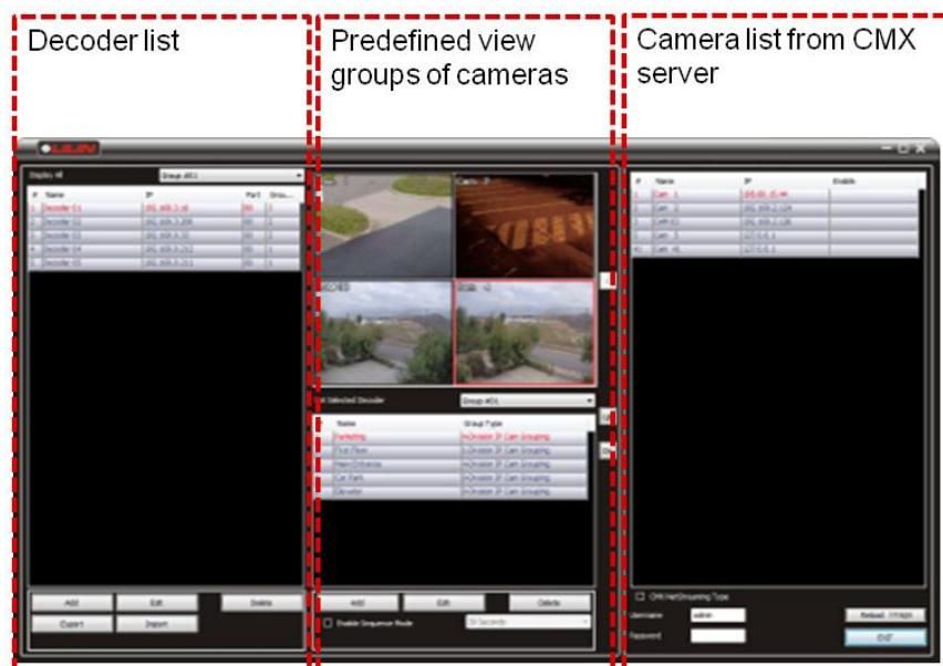
To setup video decoders, in decoder list, click Add button to add decoders with IP address, port number (default port 80), username, and password. The default username and password for video decoders are “admin” and “1111”.
