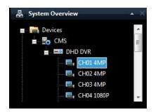
Simply click and drag the channels in to required location on the right-hand window. The camera channel should now be displayed in that location.
