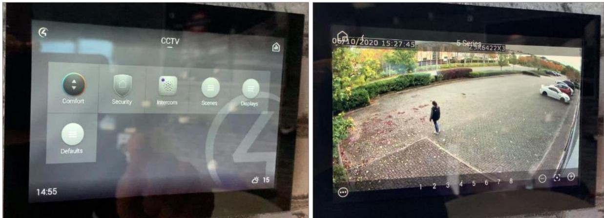
If it is a Z5 Series (auto Zoom/Focus) you can control the Zoom with the Controls at the bottom of Panel. The Preset 8 key is to Auto Focus.
