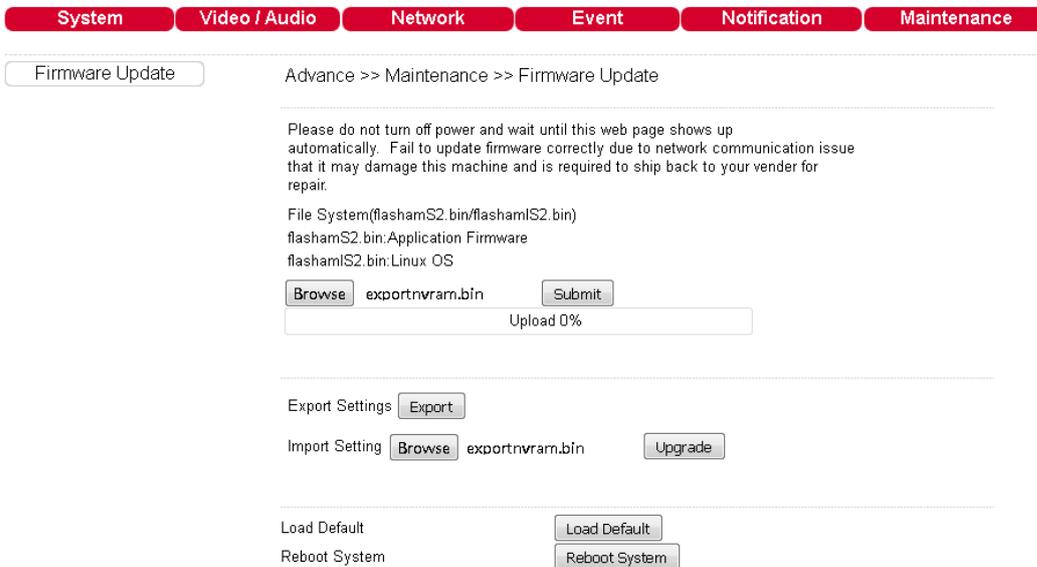
For batch configurations update for cameras, select multiple devices and click on “Firmware Update” button in IPScan. Click the “Start” button. A file dialogue box shows up for selecting the configuration file, “exportnvram.bin.” All the selected devices will get updated by the configurations.
