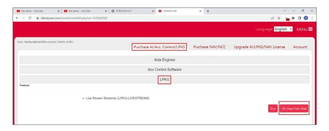
3.2.2 Input MAC adresss of your 7 series IPCAM on AI System ID column, check Live Stream Streamer (LPKG-LIVESTREAM) and click 30-Days Free Trial button.
